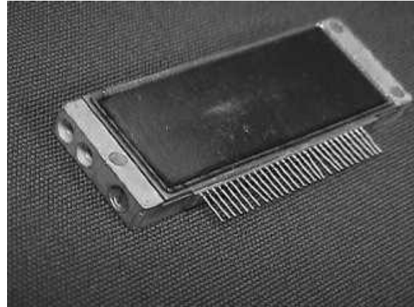
Figure 1: Ni-Au Plated Assembled AlSiC Microwave Package.
